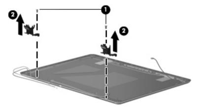
b. Remove the two microphone receivers ● from the display enclosure, and then release the microphone cable ② from the clips in the display enclosure.
